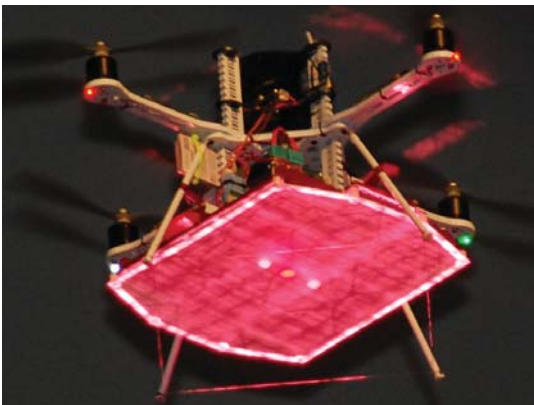
LaserMotive, LLC Example of an innovative laser power beaming system powering unmanned aerial vehicles.
