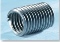
The classic design of the HeliCoil threaded insert has a tang that is used to fix the insert; this tang has to be broken off and removed during assembly. This assembly process can present issues in electrical components where a tang that is not retrieved may cause a short circuit and subsequent damage.
