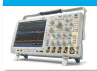
Visitors to the **SJ Electronics** stand will see the world's first mixed domain oscilloscope. This gives engineers the capability of capturing time-correlated analogue, digital and RF signals for a complete system view, in order to rapidly solve complicated design issues.
