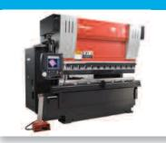
One of the 'black arts' of sheet metal bending is determining the spring-back. That's how much you over-bend to finish up with the correct angle. This can even vary between different batches of the same material. That's why the bend angle indicator, on the **Amada** latest HD series of press brakes, is such an attractive proposition.
