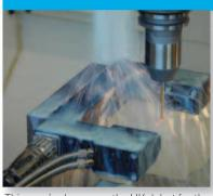
This year's show sees the UK debut for the world's first touch probe that combines digital and analogue technology from **Blum Novotest**. It is robust enough to be used in a machine tool environment. This approach promises fast detection of machining errors and a reduction in the measuring time for complex work pieces and contours.
