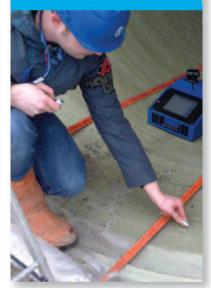
Measuring large 2D areas and 3D spaces such as the curvature of a ship's deck, or staircases are typical of the tasks that can be performed by a digital measuring system from **Prodim**. The system lends itself to reverse engineering and restoration work.
